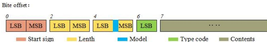
FIG 3 YDLIDAR G4 SYSTEM MESSAGE DATA PROTOCOL
