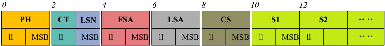
FIG 5 SCAN COMMAND RESPONSE CONTENT DATA STRUCTURE
