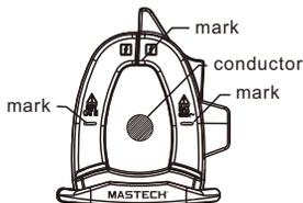
For AC current measurement, keep the conductor in the center of the clamp; otherwise the reading can deviate as much as 2.5% of actual measurement.
