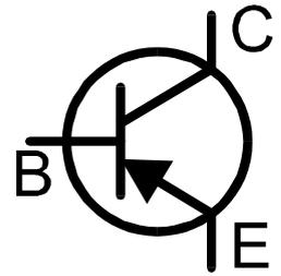
Bipolar Junction Transistors are simply “conventional” transistors, although variants of these do exist such as Darlington, diode protected (free-wheeling diode), resistor shunted types and combinations of these types. All of these variations are automatically identified by the *Atlas DCA*.
